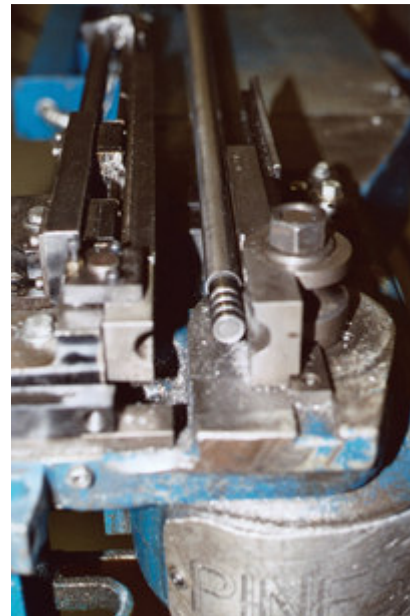
Stealth has 16 tube benders from Pines Manufacturing Inc., including one from 1946, and all of the machines have the same custom quick-change tooling designed and built by in-house staff.
