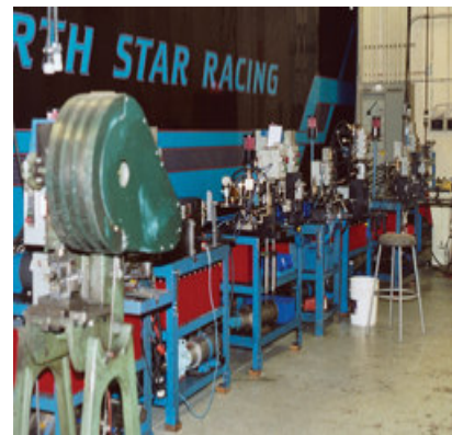
Tube fabricating machines are kept on tables that can be moved easily with a pallet jack. Operators may construct and deconstruct a workcell a couple of times per day, depending on the job size.
